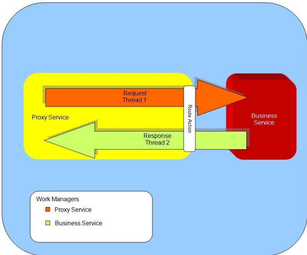
Figure 1. Threads and work managers used by a proxy service routing to a business service
