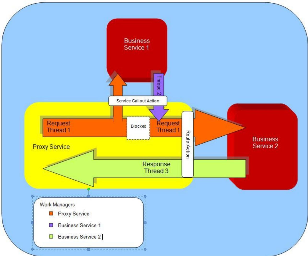
Figure 2. Threads and work managers used for a proxy service utilizing a service callout
